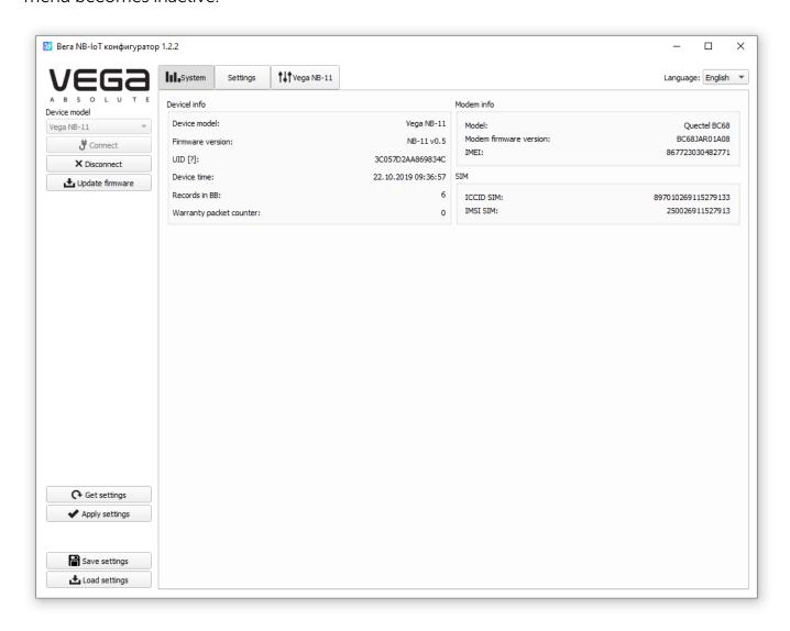
To read the settings from the device, you need to click the "Get settings" button, until this points the application will display the default settings or from the last connected device.
