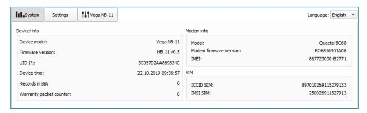
**Device info** - the configurator reads information about the device model, its firmware and automatically corrects the device's time when connected to it. In that block you can find out the number of records in the black box and the number of packets sent by the device.
